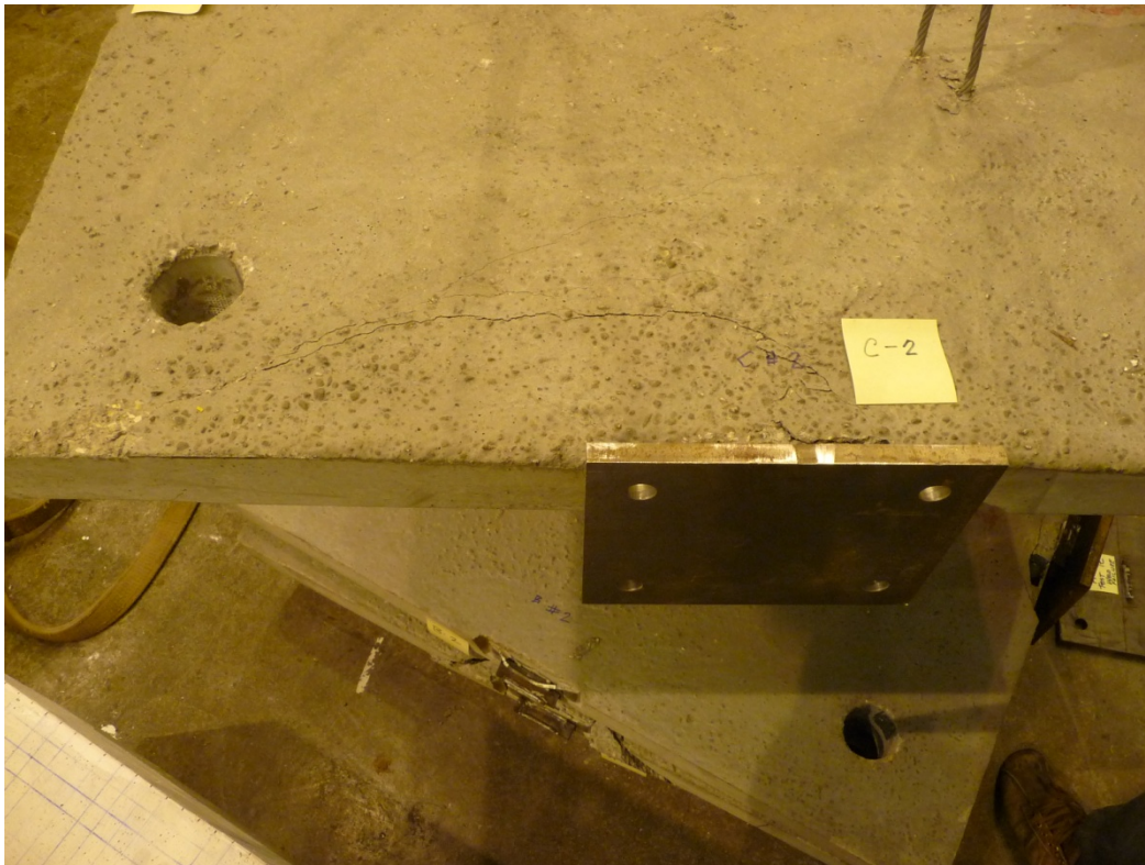
Figure 57 – Test C-2 Failure Mode – top side view
