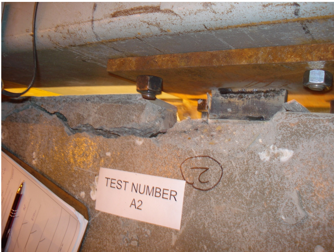
Figure 11 – Test A2: In-Plane Monotonic Shear w/ No Tension
