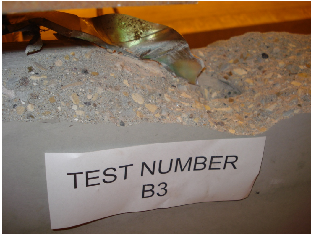
Figure 15 – Test B3: In-Plane Monotonic Shear w/ Tension
