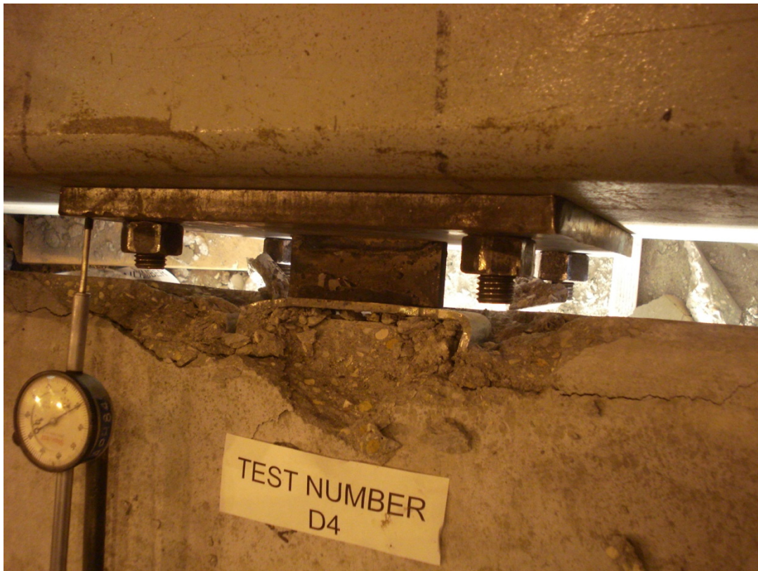
Figure 23 – Test D4: In-Plane Cyclic Shear w/ Tension
