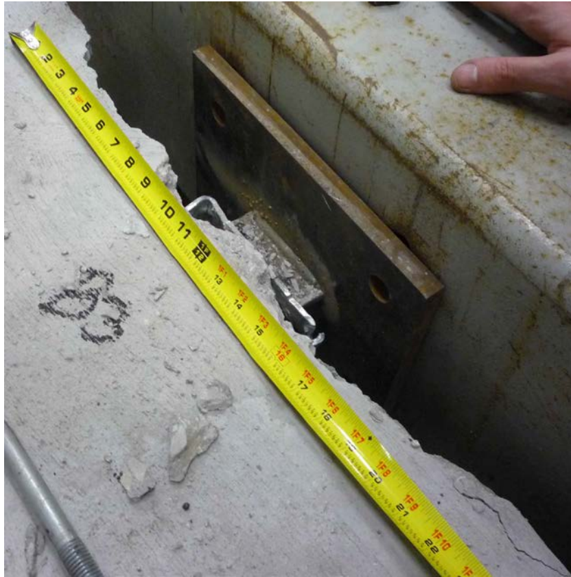
Figure 9 – Test B-3 Cyclic Shear w/ No Tension
