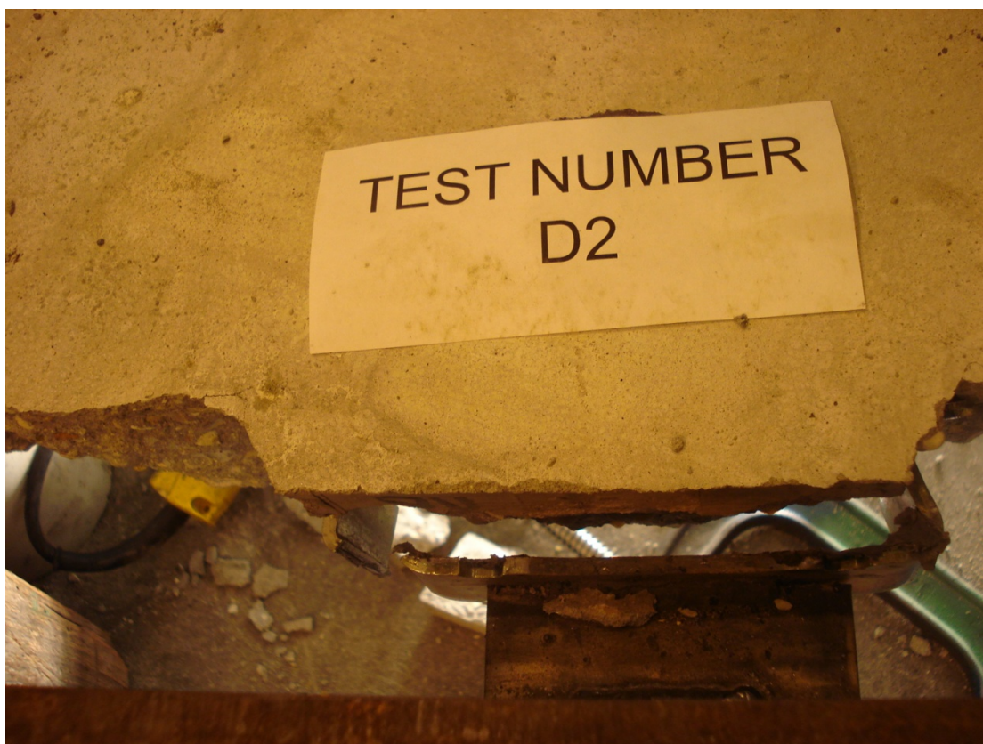
Figure 21 – Test D2: In-Plane Cyclic Shear w/ Tension
