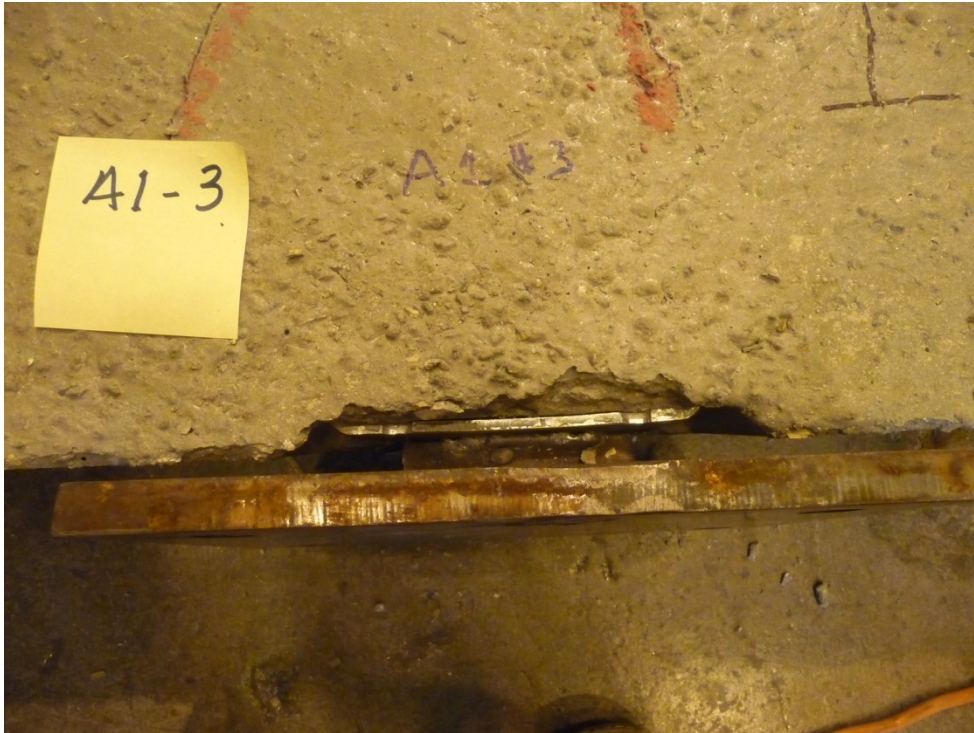
Figure 35 – Test A1-3 Failure Mode – top side view
