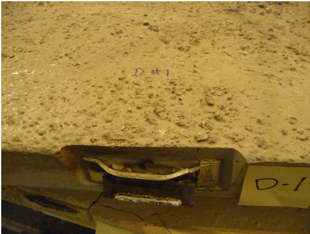
Figure 63 – Test D-1 Failure Mode – top side view
