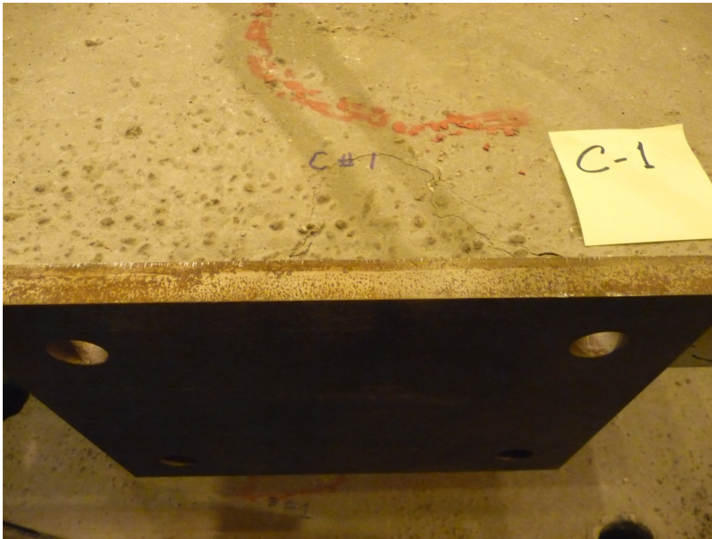
Figure 55 – Test C-1 Failure Mode – top side view
