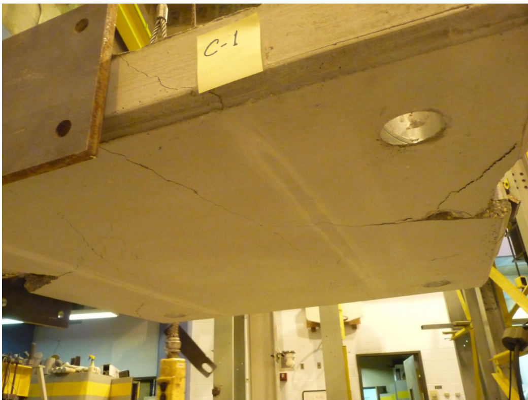
Figure 56 – Test C-1 Failure Mode – bottom side view
