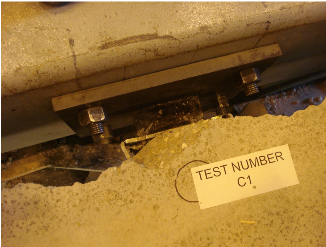
Figure 17 – Test C1: In-Plane Cyclic Shear w/ No Tension
