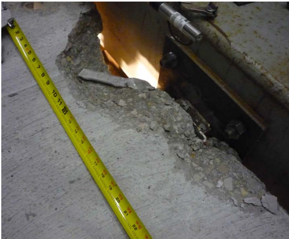
Figure 16 – Test D-2 Monotonic Shear w/ No Tension
