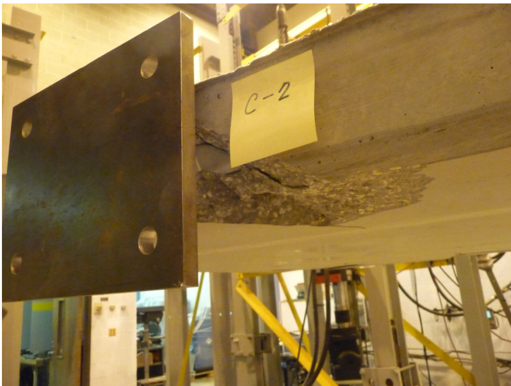
Figure 57 – Test C-2 Failure Mode – top side view
