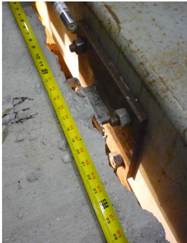
Figure 6 – Test A-4 Cyclic Shear w/ No Tension
