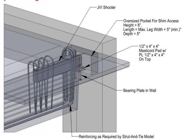
\* For a pocket with pin access on both sides of the DT leg, the pocket width should increase to Max. Leg Width + 10" min.
