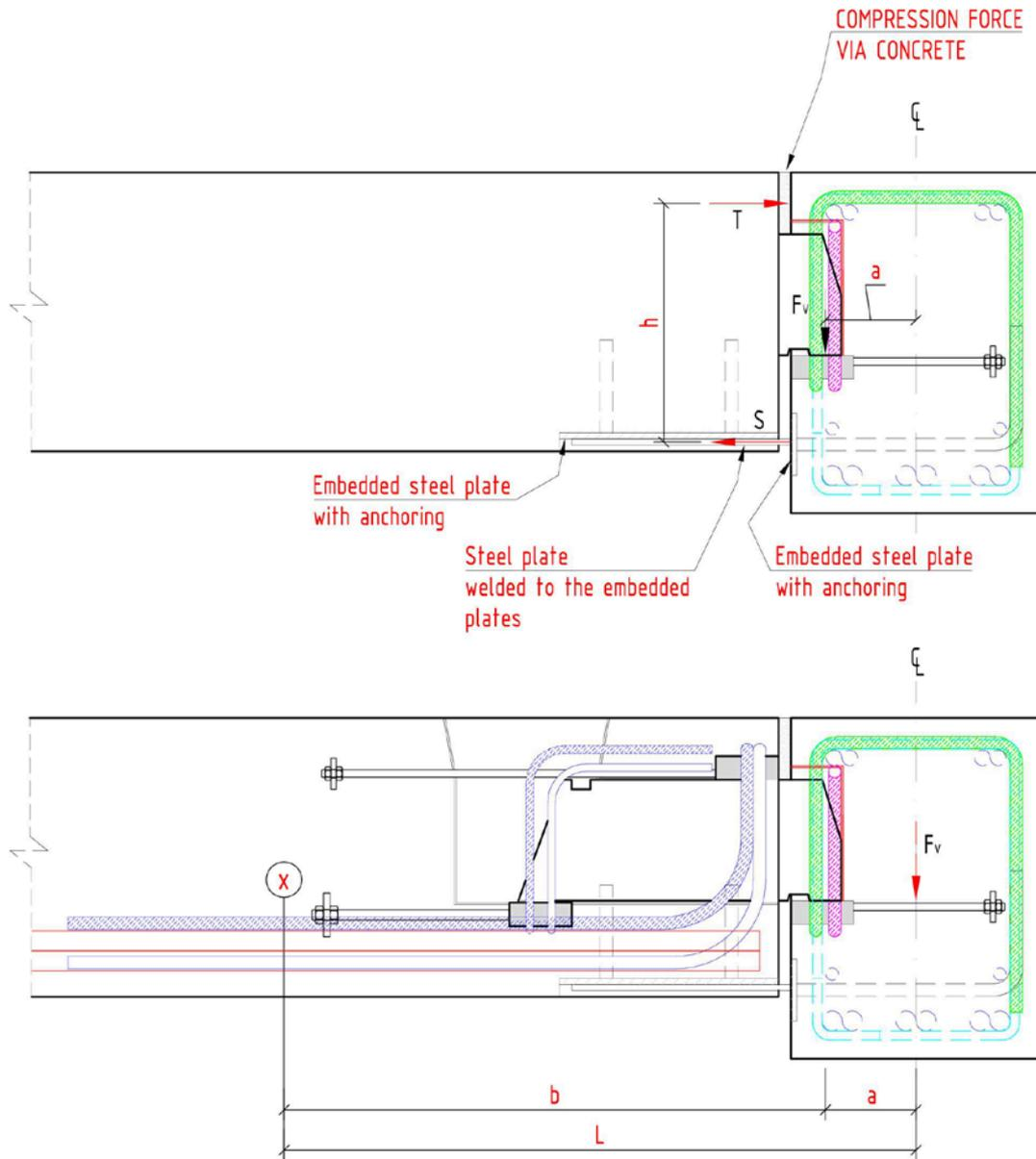
**Figure 5: Lock of torsion –main beam.**
