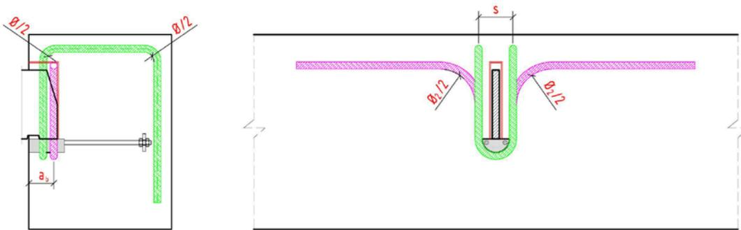
Figure 3: Bending of reinforcement.
