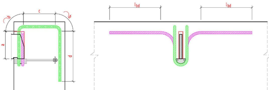
Figure 4: Anchoring of reinforcement
