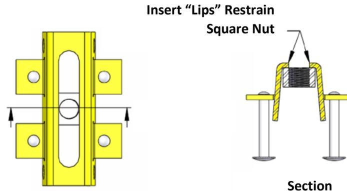
Figure 4.1.1 Insert Lips Restraining Square Nut
