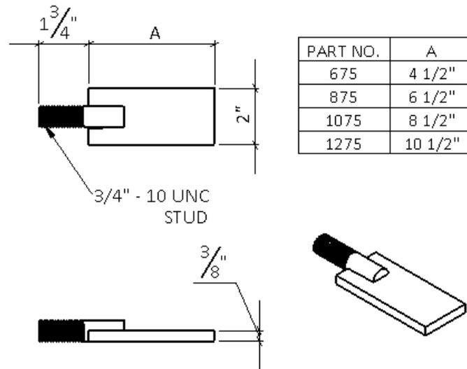
Figure 4.1.2 Strap Geometry
