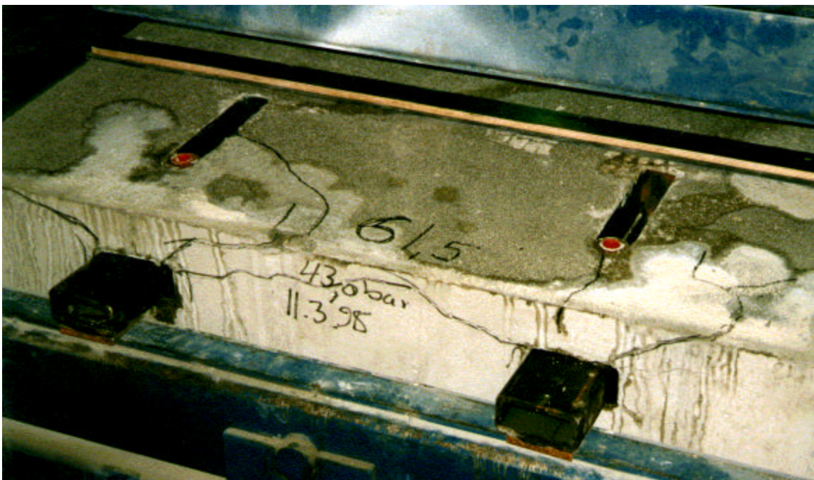
Picture 24. Test C4 at 135 kN (failure).
