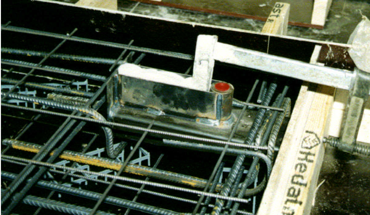
Picture 5. Reinforcement arrangement for test slabs B.
