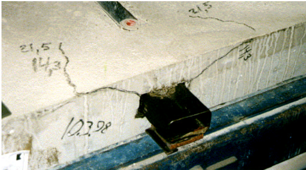
Picture 18. Test C1 at 102 kN. Notice shims at the support.
