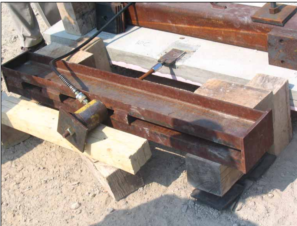
Figure A-20: Photo of perpendicular edge shear test setup.
