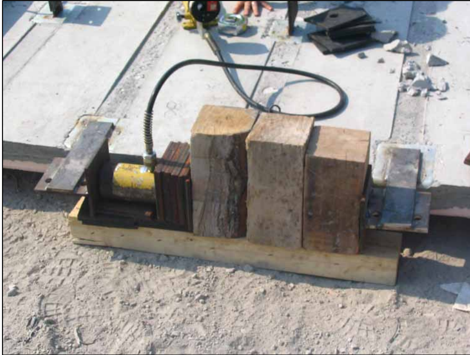
Figure A-22: Photo of parallel edge shear test setup.
