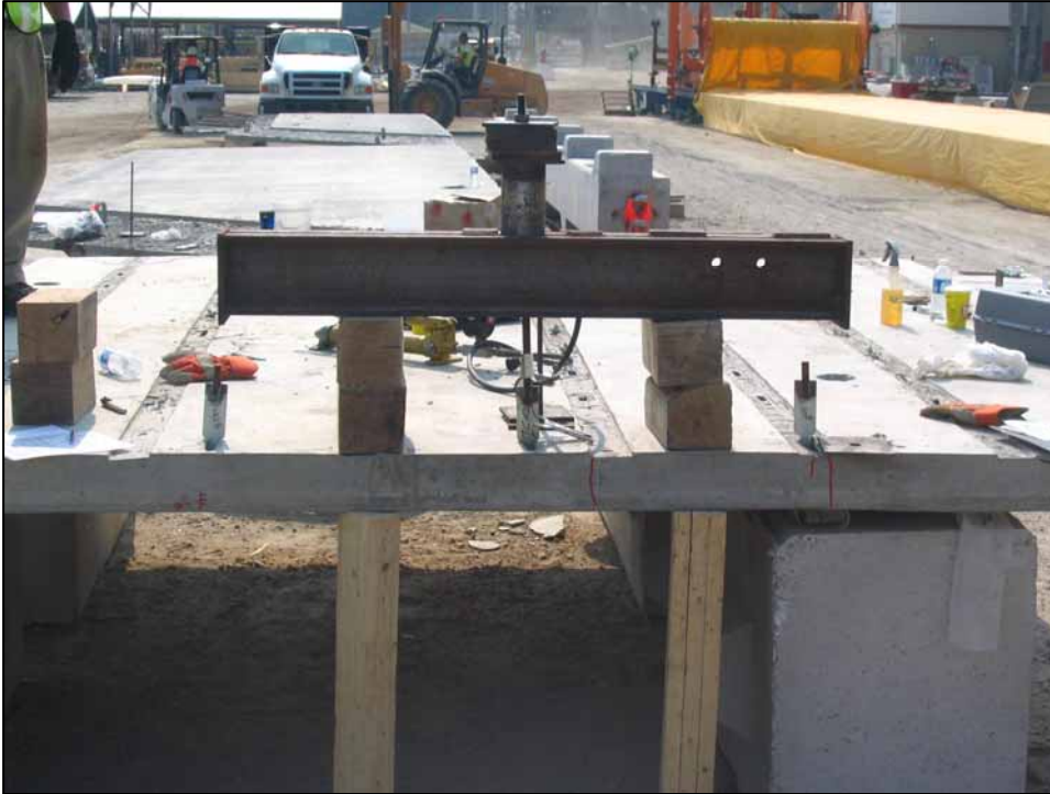
Figure A-13: Photo (front profile) of pullout test setup. Note: JVI PSA insert is being tested here, but general setup is the same for Spider plate.
