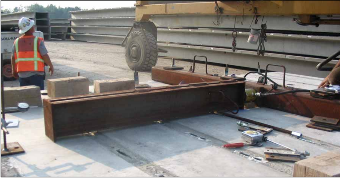
Figure A-17: Photo of lateral shear test setup.
