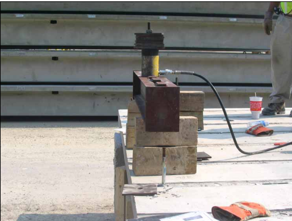
Figure A-14: Photo (side profile) of pullout test setup. Note: JVI PSA insert is being tested here, but general setup is the same for Spider plate.
