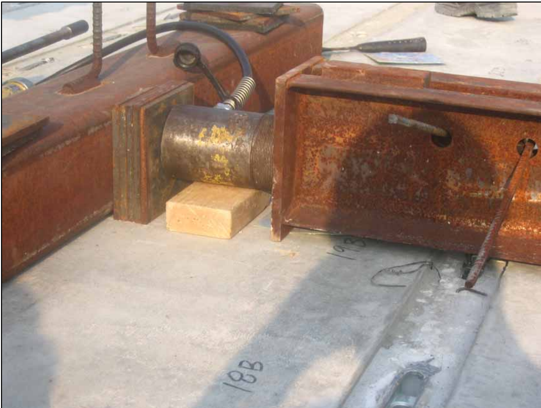
Figure A-18: Close-up photo of lateral shear test setup.
