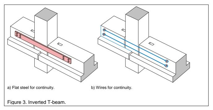
The horizontal forces are taken by either flat steel or wire straps bolted to the beam, in both cases hidden behind the end of the floor slabs. The size of the flat steel and number of bolts, as well as the number of wire straps to be determined from the magnitude of the seismic forces.
