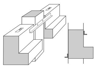
Figure 2: Clamps connected to the column.
