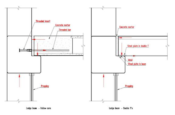
*Figure 4: Torsional moment connections. These are examples only. Other methods such as "pull out" continuity bars in the beam may also be used.*
