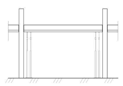
Figure 1: Temporary propping. (Illustration only, amount and location of props must be calculated and evaluated in each case)
