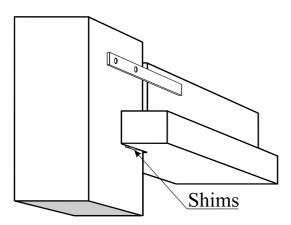
Figure 3: Beam with forked end.
