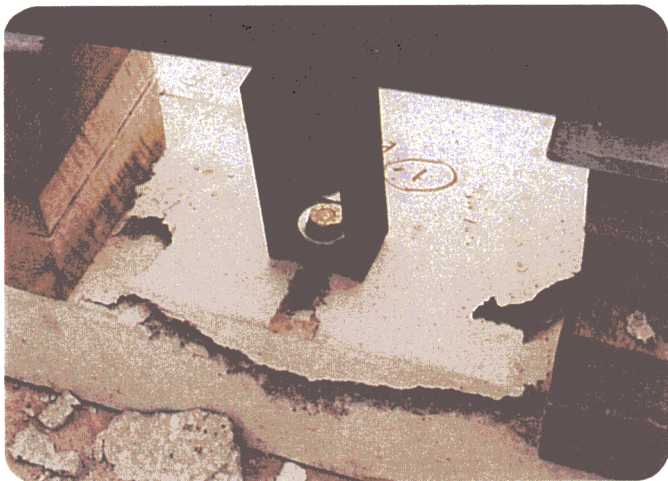
Fig. 1 6" x 2 1/2" Insert at edge - 10,200 lbs. Typical reduced concrete cone failure.
