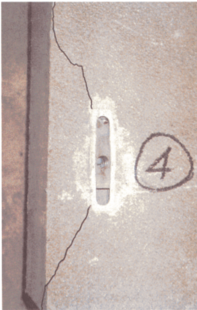
Fig. 8 Test No. 4 - (29,400 Lbs.) Corner Test with 2 Hairpins
