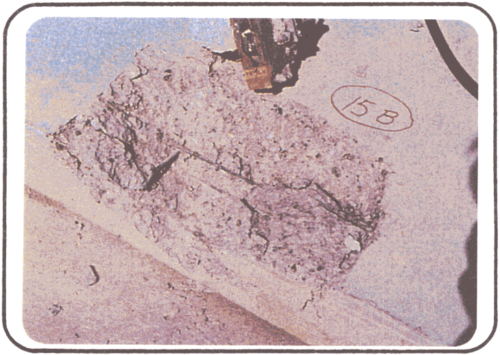
Fig. 4 4 1/2" x 4 1/2" Insert at edge, 14,100 lbs. Cone extends to base of anchors.
