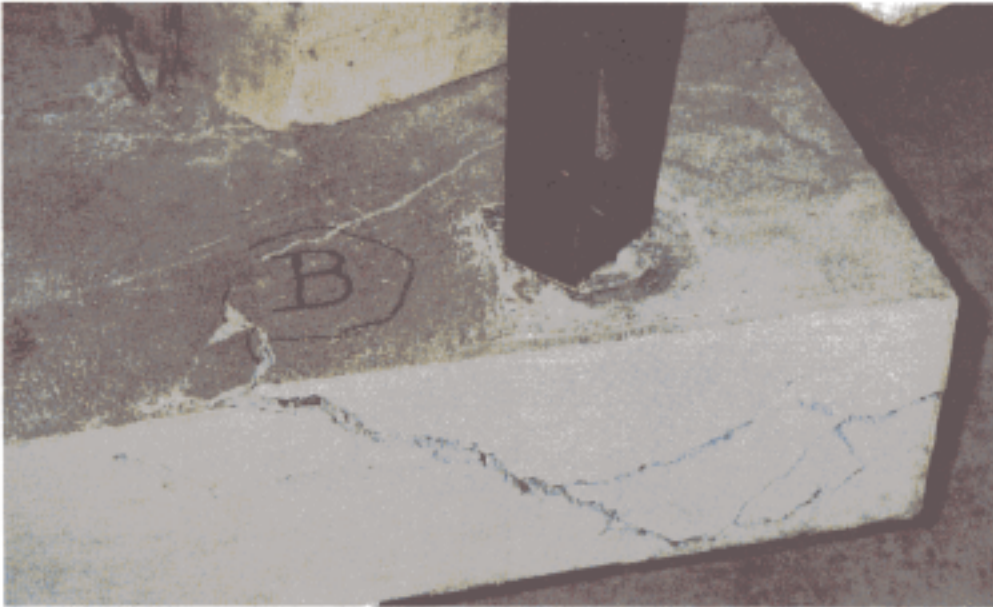
Fig. 5 Test No. B - 3/4" Ferrule at Corner - Concrete failed at 32,000 Lbs.
