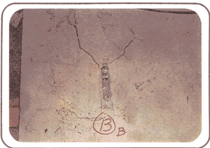
Fig. 5 Typ. 2 1/2" (12 kip) insert (Mk 6025) Test # B13 - 12,970 lbs. Load at end.
