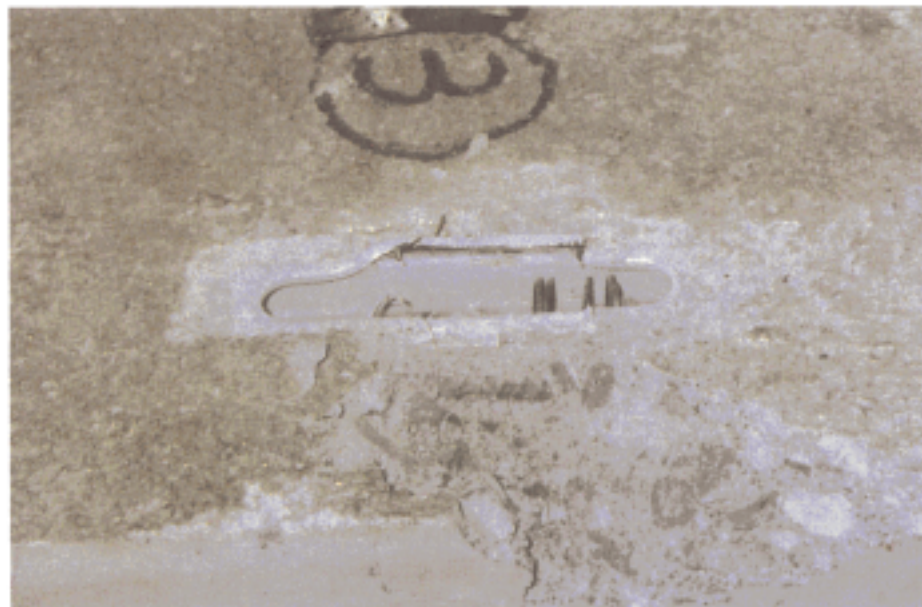
Fig. 3 Test No. 3 - (30,600 Lbs.) Corner with 2 Hairpins
