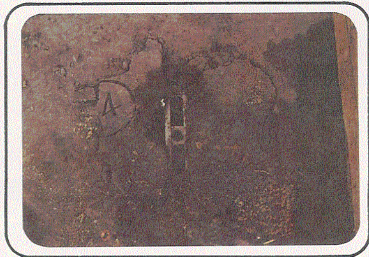
Fig. 2 Insert in 2" Concrete (Test # 14) - 9,000 lbs.
