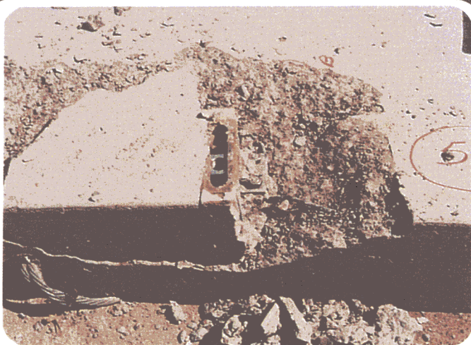
Fig. 3 4 1/2" x 3 1/2" Insert at edge, 13,800 lbs. Cone extends to base of anchors.
