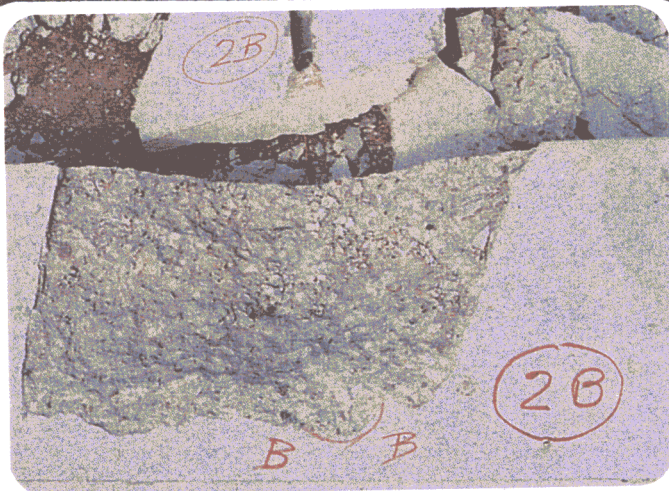
Fig. 2 4 1/2" x 2 1/2" Insert at edge, 11,500 lbs. Typical concrete cone failure. Cone extends to base of anchors.
