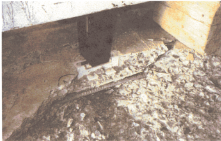
Fig. 2 Test No. 2 - (24,400 Lbs.) No stepped hairpins
