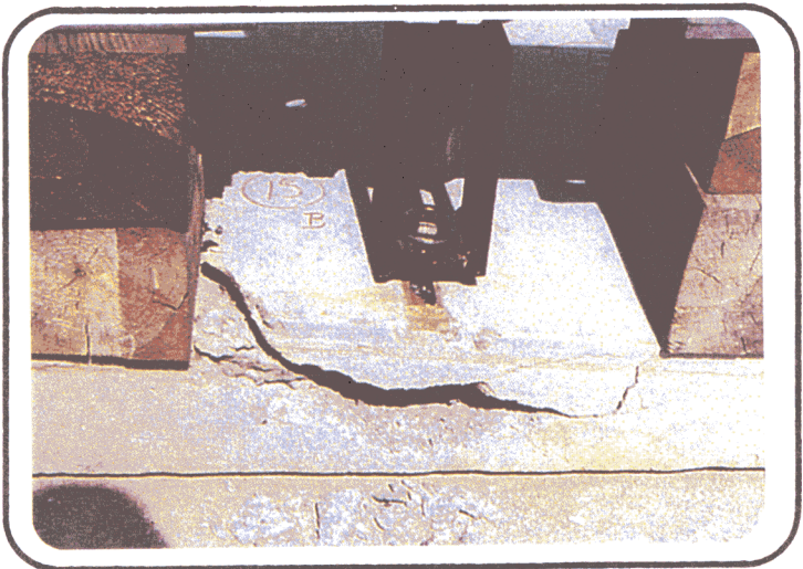
Fig. 5 4 1/2" x 4 1/2" Insert at edge. 14,100 lbs. Typical concrete failure. Insert intact.
