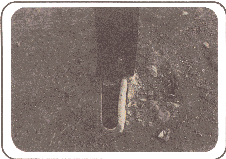
Fig. 3 Typical failure (Test # 1) e = 1 \frac{1}{2}" 17,900 lbs.
