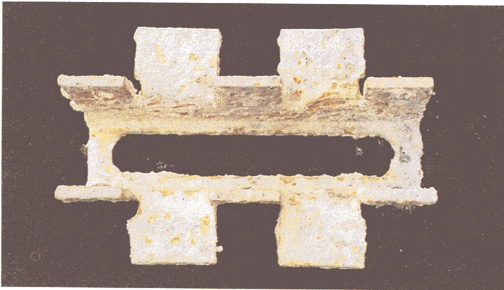
Fig. 5b PSA Insert (Bottom) Hot Dip Galv. Finish after 648 hours
