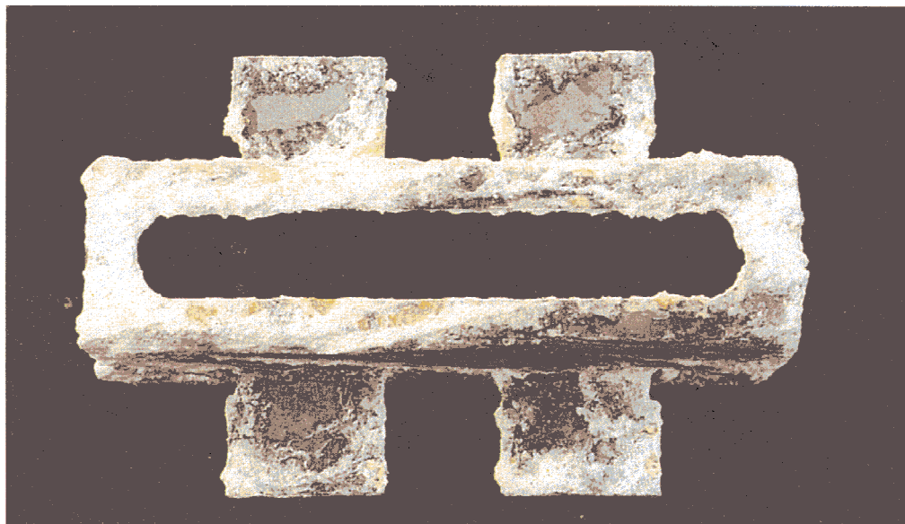
Fig. 5a PSA Insert (Top) Hot Dip Galv. Finish after 648 hours
